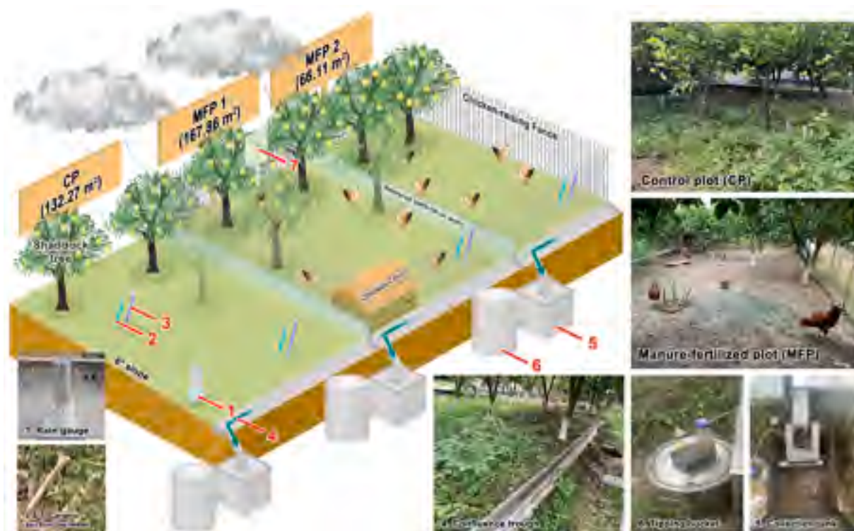
Fig. 1. Schematic picture of experimental plots with rainfall monitoring and surface runoff sampling facilities (CP, control plot; MFP1/2, parallel manure-fertilized plots).
