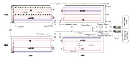
**Figure 1.** Experiment layout. CW and RW are Fresh water and Reclaimed water. DSI and FUI are Subsurface drip irrigation and Furrow irrigation. FI and APRI are Full irrigation and alternate partial root-zone irrigation.
