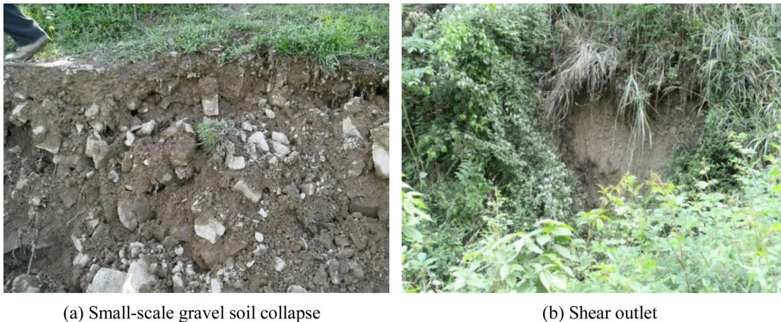
Fig. 10 Small-scale gravel soil collapse and shear outlet in front of the slope. a Small-scale gravel soil collapse. b Shear outlet
