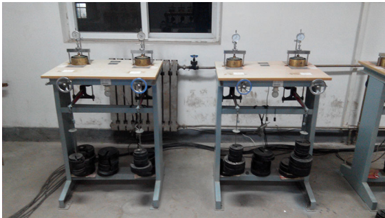
Fig. 1 Some specimens in the creep tests
