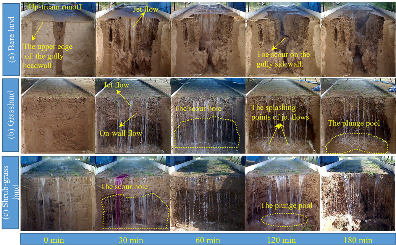
FIGURE 4 Gully head retreat processes driven by hydraulic erosion over time under different land use/cover types [Colour figure can be viewed at wileyonlinelibrary.com ]
