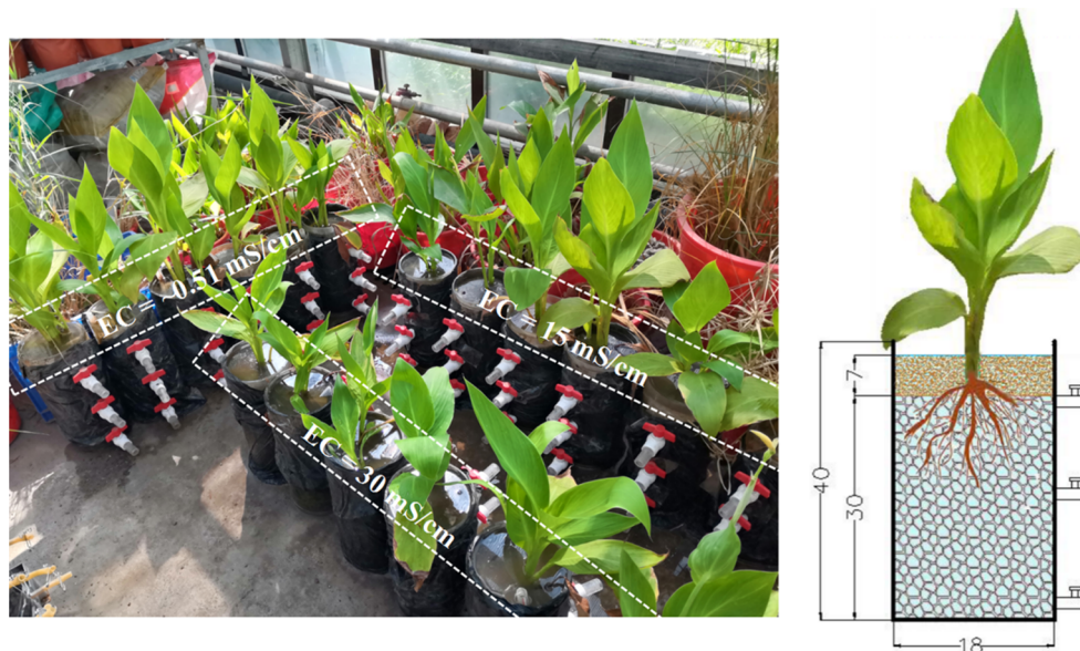
Fig. 1. A photo and schematic diagram of CW microcosms (Unit: centimeter). EC: electrical conductivity.
