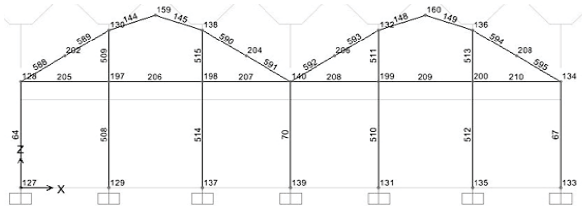
FIGURE 2 The numbering of Gothic Roofed Greenhouse Construction Elements
