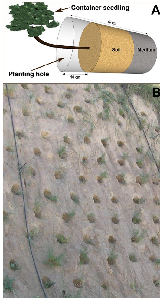
Figure 3. Schematic of the method of deep-planting container seedlings (A) and a photograph of a slope after completion (B)
