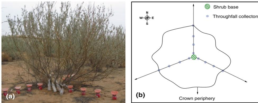
Fig. 2 Photograph (a) and schematic layout (b) showing throughfall collection for *C. korshinskii*
