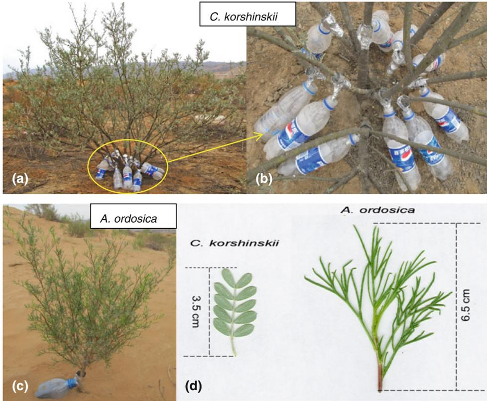
Fig. 1 Photographs showing the stemflow collection systems for *C. korshinskii* and *A. ordosica* and their leaf characteristics
